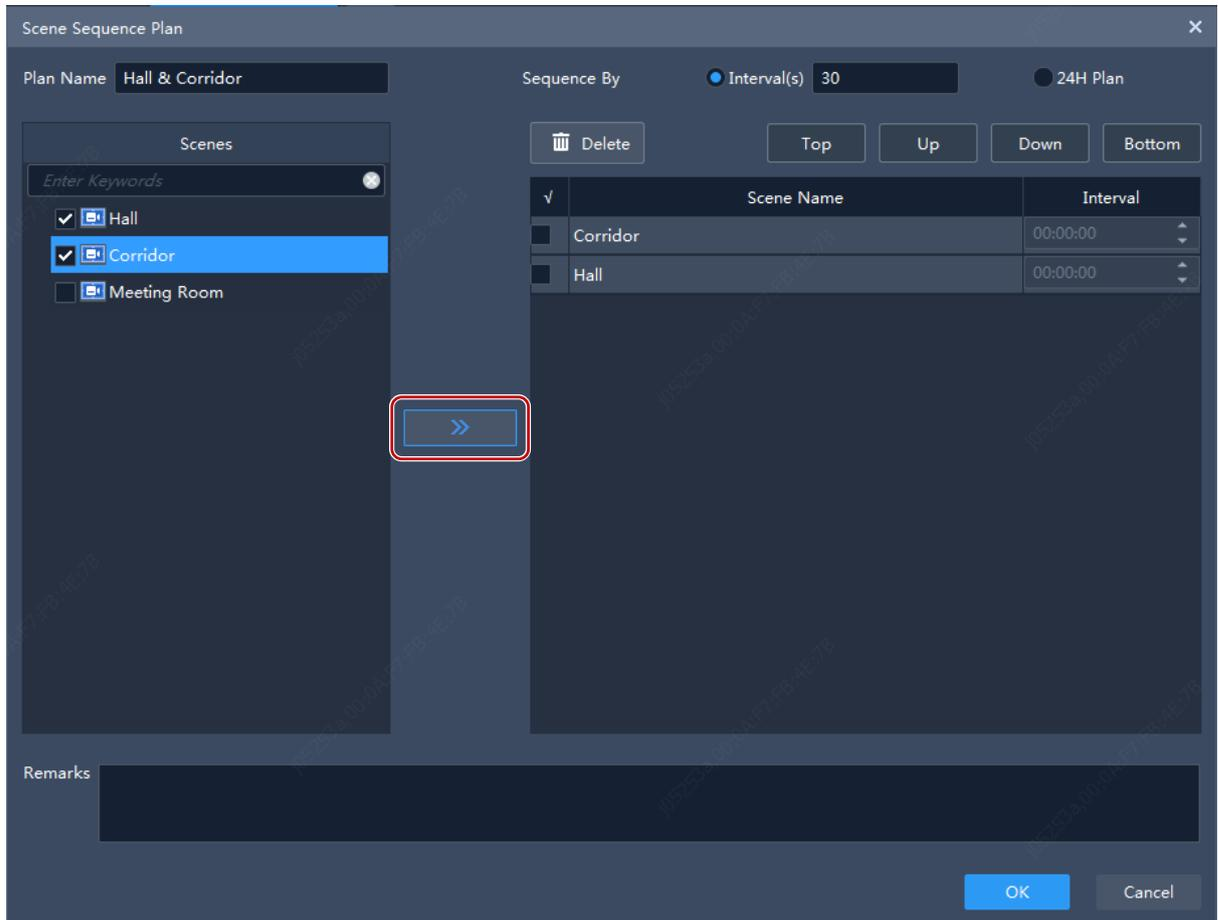
4. Set the sequence mode. You may choose to sequence by time interval or configure a 24-hour sequence plan.
