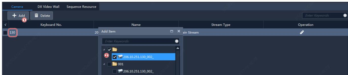
3. On the **DX Video Wall** tab, click **Add** to add a video wall. You need to configure video wall first. See [Video Wall](#) for details.
