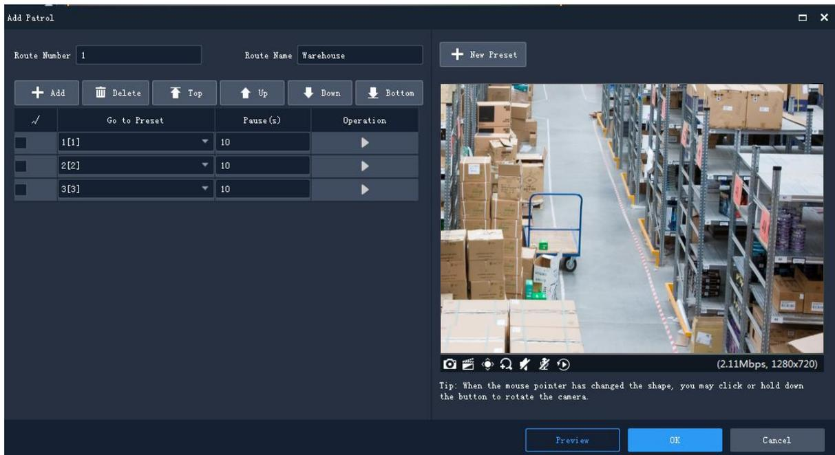
3. Click **Add**, select a preset, and set the length of time that the camera stays at this position. Repeat this step to all the necessary presets.
