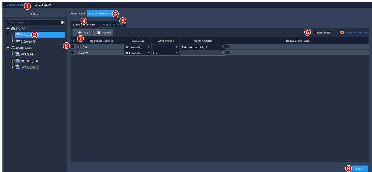
1. Click a tab according to the alarm type you want to configure. Take **Camera Alarm** for example.
