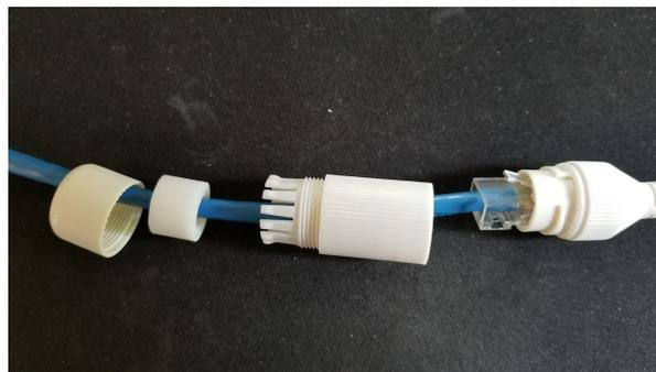
Step 5. Connect everything together and tighten down the compression cup until the barrel gasket is tight around the Cat5 cable.
